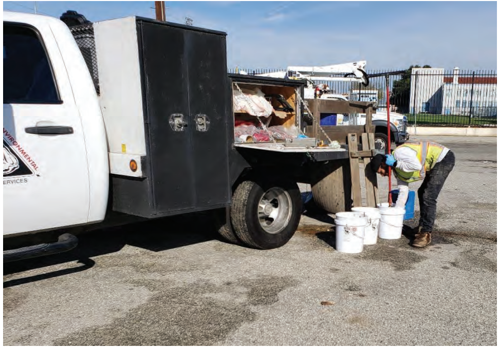
Photograph 29: Worker decontaminating hand auger between soil borings to avoid contamination.
