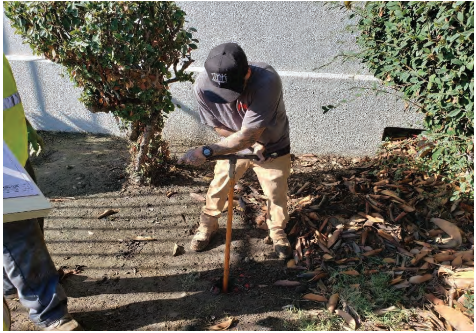
Photograph 15: Worker hand-augering soil boring for lead analysis on Compton High School main campus.
